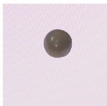
Vistrol COB After Collision Test (>10kg, ~1m Height)
